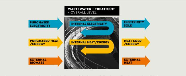
A wastewater treatment plant's energy flows. Drinking water and the pipe network share the same figure, however, without the 2 lowermost biomass arrows.
